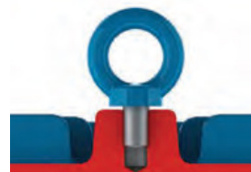
Figure 4.2 - Incorrect tightening of the eyebolt
