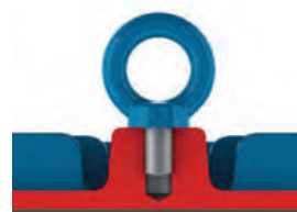
Figure 4.1 - Correct tightening of the eyebolt
