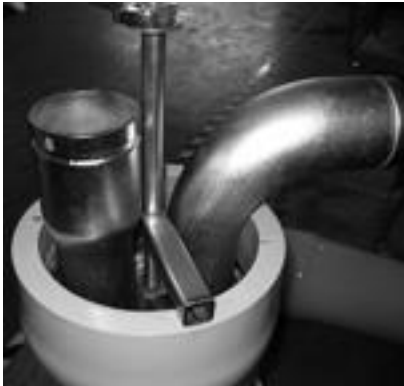
Figure 8.4 – Extract port bearing plate subassembly with puller tool
