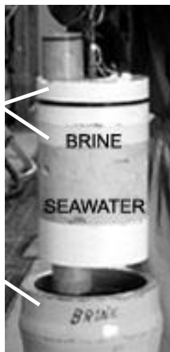
Figure 8.7 – Mark rotor subassembly to preserve correct orientation
