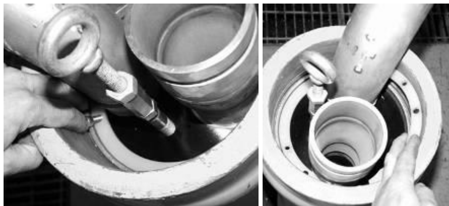
Figure 8.2 – Remove 5/16-inch socket cap screws and remove the securing ring
