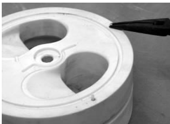
Figure 8.9 - Insert dowel pins into endcovers
