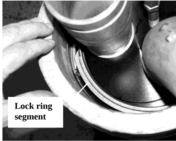
Figure 8.16 – Insert 3-part segmented lock ring
